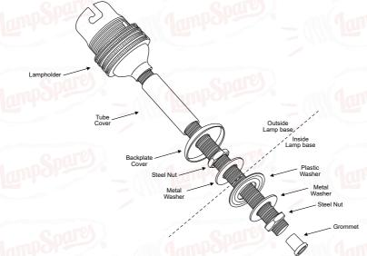
**Step 2:** Ensure the threaded rod is sticking out the top of the vase enough for the cover and lampholder to fit, below is a quick guide on the correct lengths.
