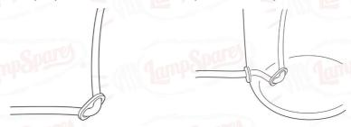
**Step 4:** Wire the lampholder connection unit and carefully push the connection unit into the lampholder's base.
