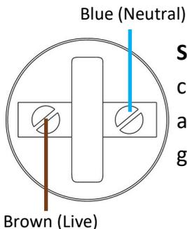
**Step 5:** Connect the wires to the Lampholder connection unit, It does not matter which way around the Live (Brown) and the Neutral (Blue) go.
