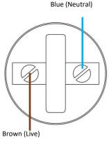
**Step 5:** Connect the wires to the Lampholder connection unit, It does not matter which way around the Live (Brown) and the Neutral (Blue) go.
