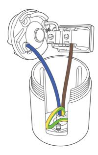
**Step 4:** Sit the switched insert carefully into the cap. Carefully screw the skirt onto the cap which will hold the insert in place. This will click as its tightened up which is the locking device.
