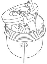
**Step 4:** Sit the insert carefully into the cap so the cord can travel in and out the hole freely. Please see picture to the left.
