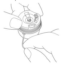
**Step 6:** Carefully screw the lampholder skirt onto the lampholder cap which will hold the insert in place. This will click as it's tightened up, which is the locking device. If you need to open the lampholder depress the barb whilst turning the skirt anti-clockwise.
