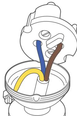
**Step 5:** Carefully push the connection unit into the Lampholder's bottom section.
