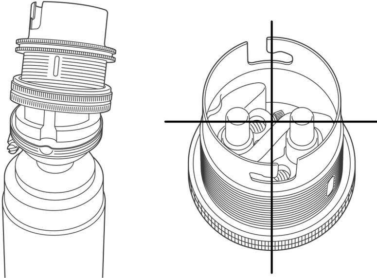
**Step 7:** Once the lampholder has been installed and aligned correctly, finally using a slotted screwdriver tighten the black nylon screw up on the side entry cord grip, ensuring the cable cannot be pulled out of the lampholder.
